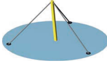
Figure 5.2: A single rod with three strings
