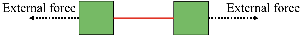
Figure 1.6: Two rigid bodies and a single string that do not constitute a tensegrity configuration
